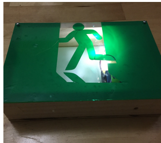
William created an emergency exit light that automatically turn on when it is dark.
