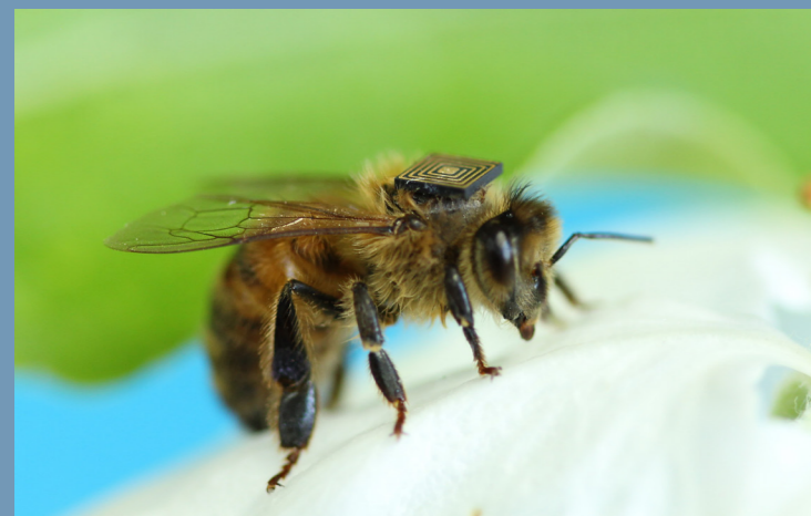
Bee with a backpack... of the sensor variety. From CSIRO Case study - Swarm sensing: tiny technology creates a buzz
